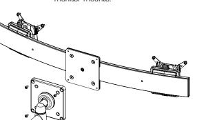
Slide mount onto rail with tab in up position
