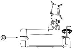
Position Arm so it is parallel to desk surface. Turn bolt clock wise for lighter monitors.
